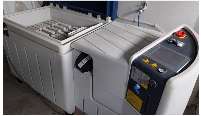
Fig. 10. Testing the durability in chloride corrosion
