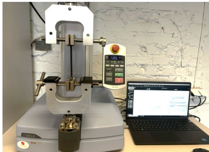
Fig. 2. SHIMADZU testing machine with recording equipment used for tensile testing
