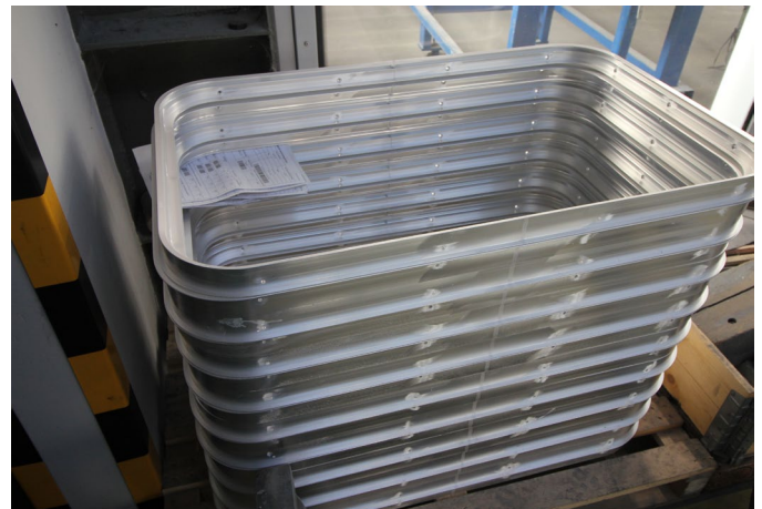
Fig. 2. The window frame is made of tested aluminium alloy
