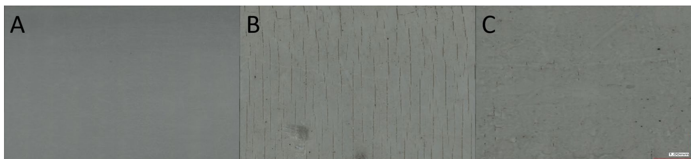
Fig. 5. Surface of POM samples: primary sample (A), sample aged in natural conditions (B), sample aged in accelerated conditions 750 h (C)
