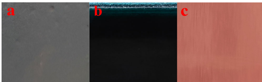
Fig. 8. Images of after improvements of anode dissolution (a), electrolyte (b) and cathode (c) of low arsenic anode respectively, 65^\circ\text{C} , at high current density of 300 \text{ A/m}^2
