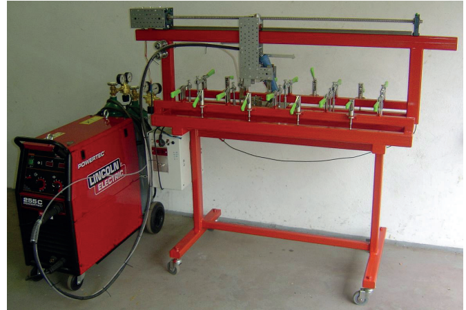
Fig. 5. Apparatus for welding with micro-jet cooling
