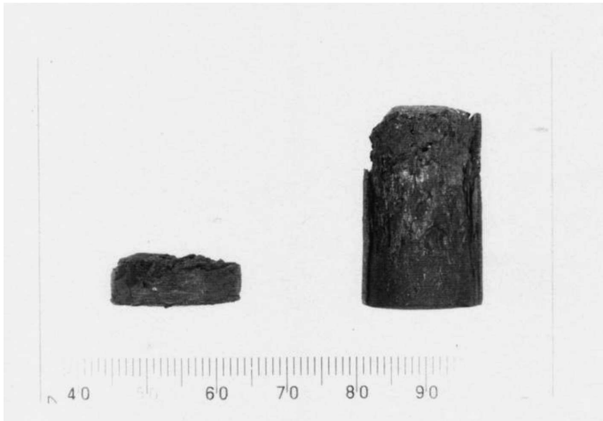
Fig. 2. Outer views of as-synthesized (right) and compacted specimens (left)
