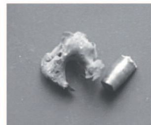
Fig. 6. Typical destruction of ceramic components (a) and bullet (b) (fragments of bullet core and shell)
