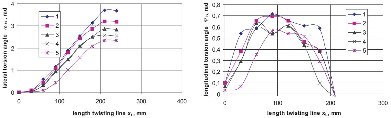
Fig. 4. Dependence twisting parameters piercing and spreading process from length pipe for  $d_g = 46$  mm,  $\beta = 10^\circ$  and variable advances plug piercing  $m$ : 1 – 16 mm, 2 – 22 mm, 3 – 28 mm, 4 – 34 mm, 5 – 40 mm
