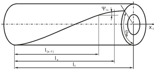
Fig. 2. Schema twisting line formed in outside layers pipe
