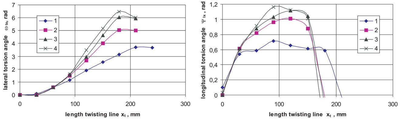
Fig. 5. Dependence twisting parameters piercing and spreading process from length pipe for  $m = 16$  mm,  $\beta = 10^\circ$  and variable diameter plug piercing  $d_g$ : 1 – 46 mm, 2 – 48 mm, 3 – 50 mm, 4 – 52 mm
