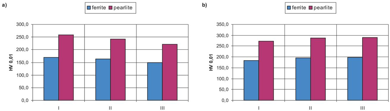
Fig. 10. Microhardness of the samples for variable advance plug piercing (m), barrel type roll pass design: a) sample no 16 m = 16 mm; b) sample no 17 m = 40 mm; I – external part, II – middle part, III – internal part cross-section tube
