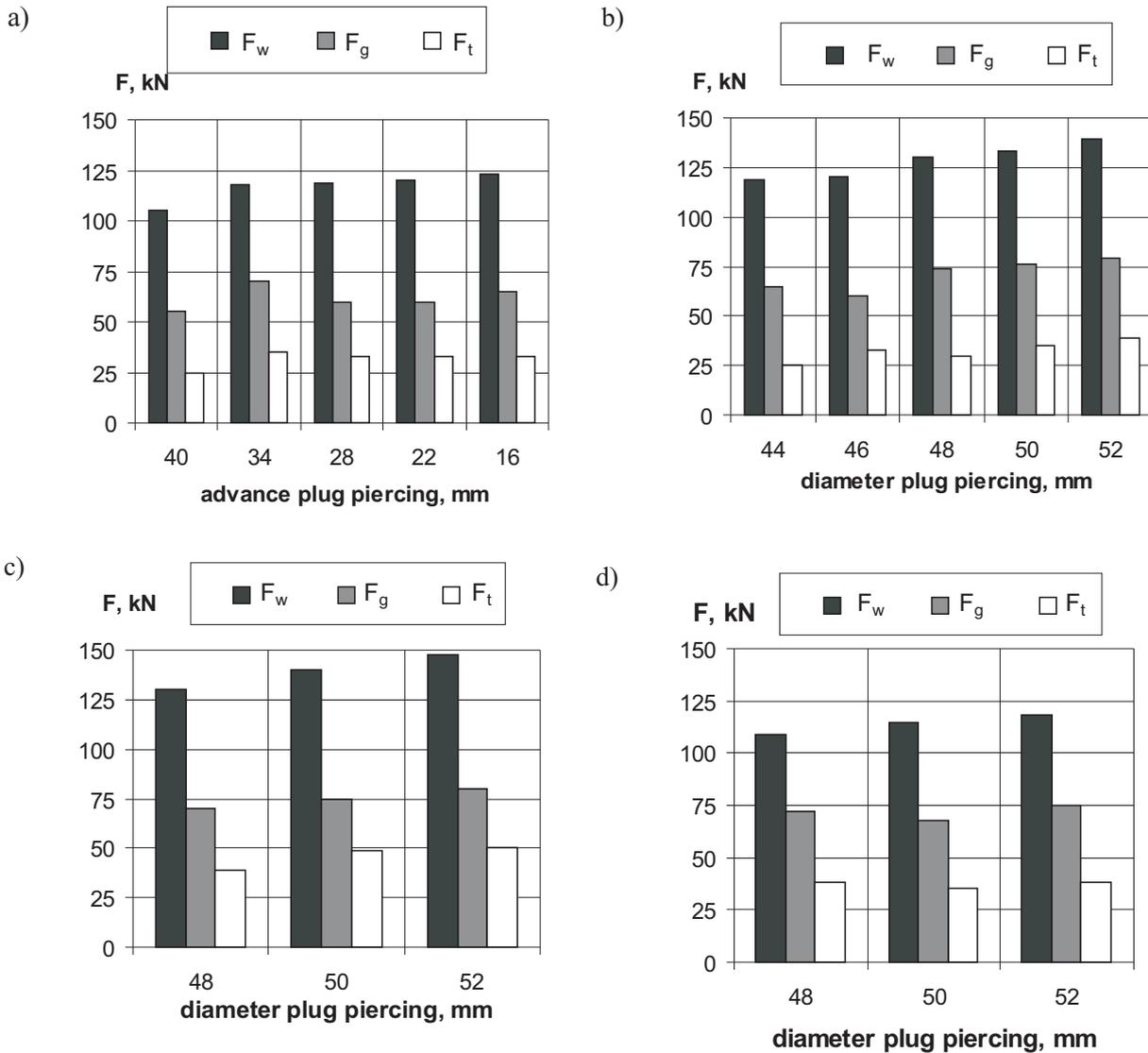
Fig. 3. Powers parameters piercing and spreading process, were:  $F_w, F_g, F_t$  – roll, plug and disc guide force: a)  $m = 40 \div 16$  mm,  $d_g = 46$  mm; b)  $m = 22$  mm,  $d_g = 44 \div 52$  mm; c)  $m = 16$  mm,  $\beta = 10^\circ$ ; d)  $m = 16$  mm,  $\beta = 12^\circ$
