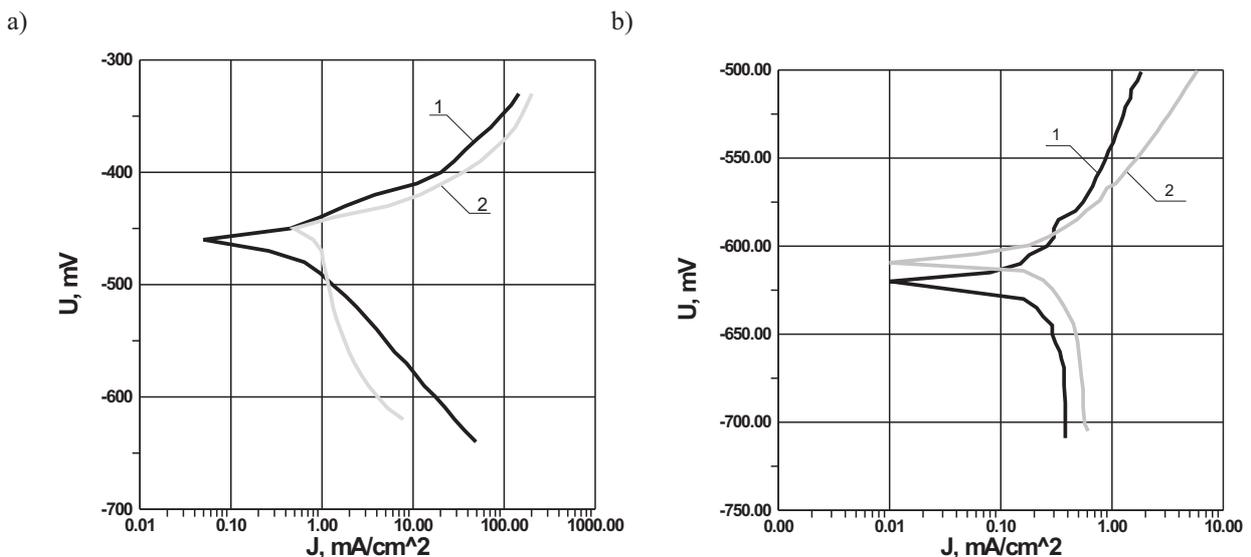
Fig. 11. Potentiostatic polarization curves for 1 – full annealing sample and 2 – pipe subjected to skew rolling mill in range  $\pm 150$  mV from potential corrosive in: a) electrolytic solution of 5%  $H_2SO_4$  and b) in sea water [17, 18]
