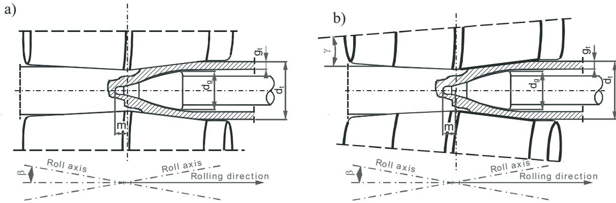
Fig. 1. Shape and position of the working tools in the strain area, roll pass design: a) of barrel type and b) of cone type, of the skew piercing-spreading rolling mill was applied
