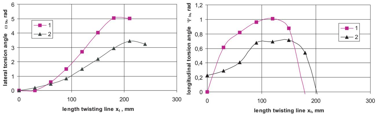
Fig. 6. Dependence twisting parameters piercing and spreading process from length pipe for  $m = 16$  mm,  $d_g = 48$  mm and variable feed angle  $\beta$ : 1 –  $10^\circ$ , 2 –  $12^\circ$
