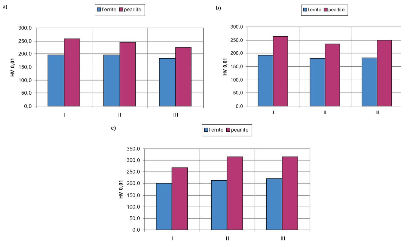
Fig. 9. Microhardness of the samples for variable plug piercing diameter ( $d_g$ ): a) sample no 1  $d_g = 48$  mm; b) sample no 2  $d_g = 50$  mm; c) sample no 3  $d_g = 52$  mm; I – external part, II – middle part, III – internal part cross-section tube
