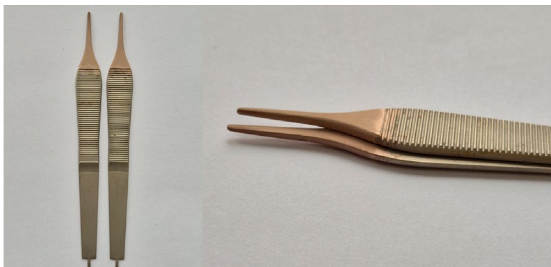
Fig. 5. Copper-coated nickel tweezers. The coatings were produced under optimum conditions: 70 \pm 5^\circ\text{C} for 30 minutes in a solution containing 0.55 \text{ M NaH}_2\text{PO}_4 \cdot \text{H}_2\text{O} at pH 9.5
