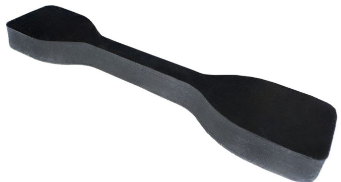
Fig. 5. Photo of the sample after cutting by machining using a CNC milling machine
