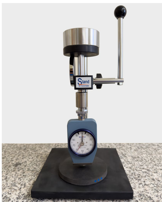
Fig. 3. Hardness tester Teclock Shore A
