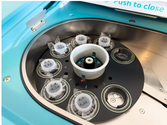
Fig. 2. Samples placed in the SPECTRO XEPOS spectrometer
