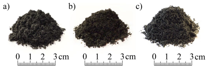
Fig. 1. Test samples in the form of dust: a) NBR rubber; b) EPDM rubber; c) SBR rubber
