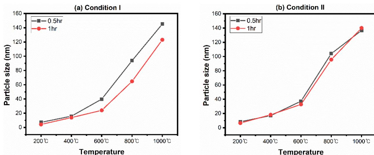
Fig. 4. Comparison of particle size in heat-treated samples under (a) Condition I and (b) Condition II
