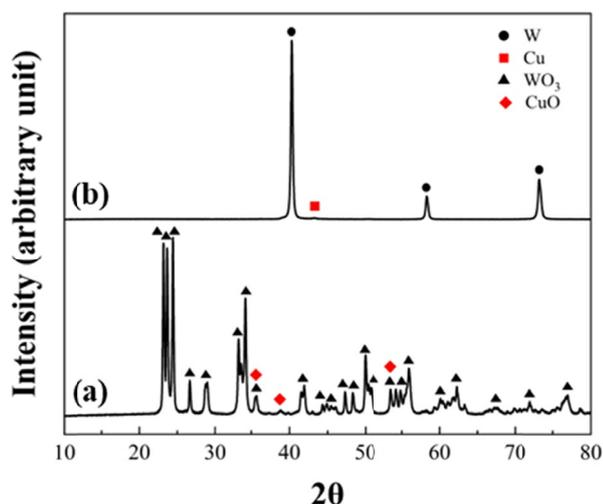
Fig. 2. XRD profiles for the powder mixture of commercial  $\text{WO}_3$  and copper nitrate after (a) calcination at 300°C in air and (b) reduction at 800°C in hydrogen atmosphere
