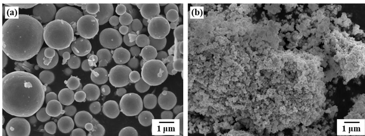
Fig. 1. SEM micrographs of calcined composite powders using (a) USP and (b) commercial  $\text{WO}_3$  as raw powders
