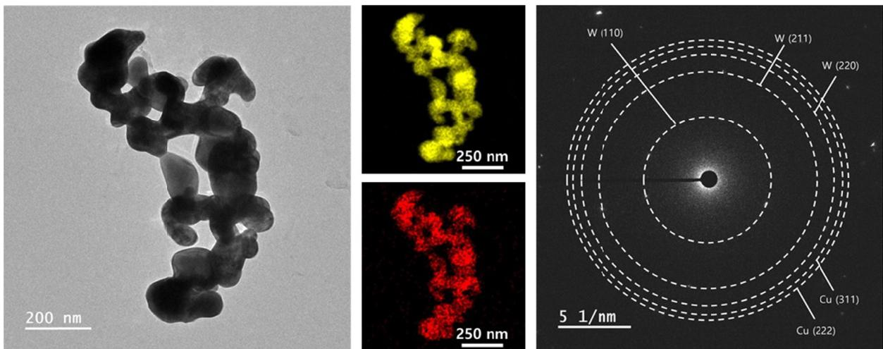
Fig. 4. TEM-EDS-SAED results of hydrogen-reduced W-5 wt.% Cu composite powder
