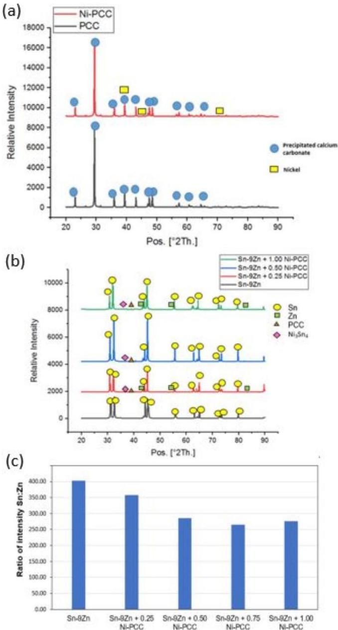
Fig. 2. (a) X-ray diffraction of plain PCC and Ni-PCC; (b) XRD curve composite solder Sn-9Zn + xNi-PCC ( $x = 0.25, 0.50$  &  $1.00$  wt.%); (c) ratio intensity of Sn to Zn of Sn-9Zn and composite solder Sn-9Zn + x Ni-PCC ( $x = 0.25, 0.50$  &  $1.00$  wt.%)
