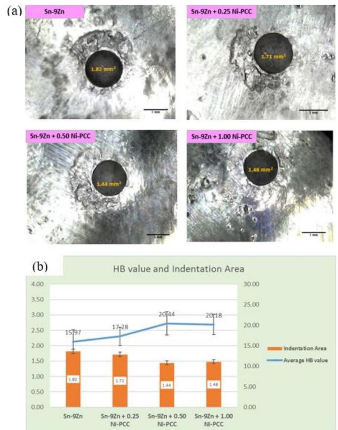
Fig. 5. (a) Image of indentation of composite solder Sn-9Zn + xNi-PCC ( $x = 0.25, 0.50$  &  $1.00$  wt.%) after Brinell Test; (b) Average HB value and Indentation Area of composite solder Sn-9Zn + x Ni-PCC ( $x = 0.25, 0.50$  &  $1.00$  wt.%) after Brinell Test
