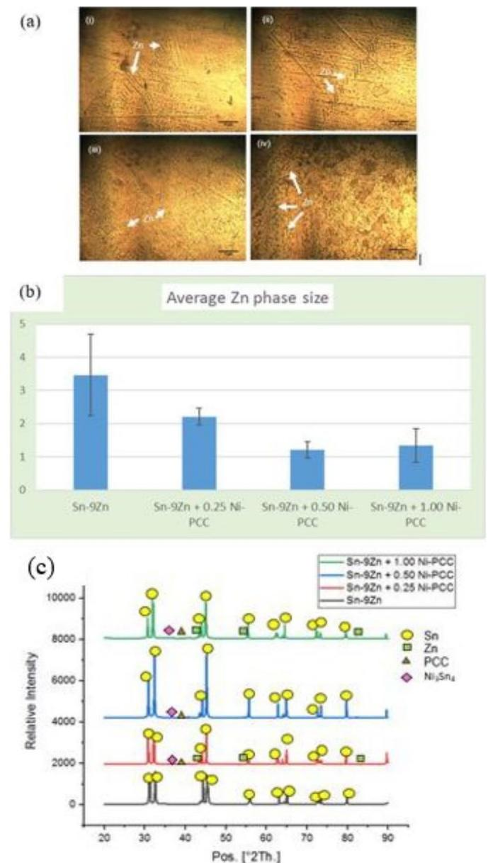
Fig. 3. (a) Microstructure of composite solder Sn-9Zn + xNi-PCC (i)  $x = 0$ , (ii)  $x = 0.25$ , (iii)  $x = 0.50$ , (iv)  $x = 1.00$  wt.%; (b) Average size of Zn phase of composite solder Sn-9Zn + xNi-PCC ( $x = 0, 0.25, 0.50$  &  $1.00$  wt.%)
