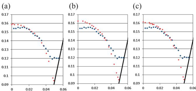
Fig. 5. Profile of the liquid metal surface for CFD solution (red points) and measurement results (blue points) inside a crucible space (in mm) for different turbulence models: (a)  $k-\epsilon$ , (b)  $k-\omega$  and (c) transition SST
