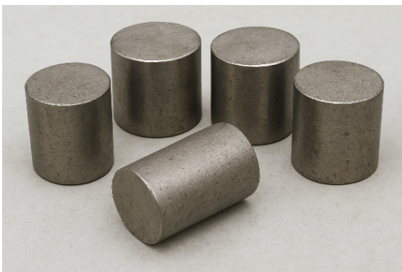
Fig. 3. SiC and Gr particles reinforced fabricated Al 7075 composite specimens
