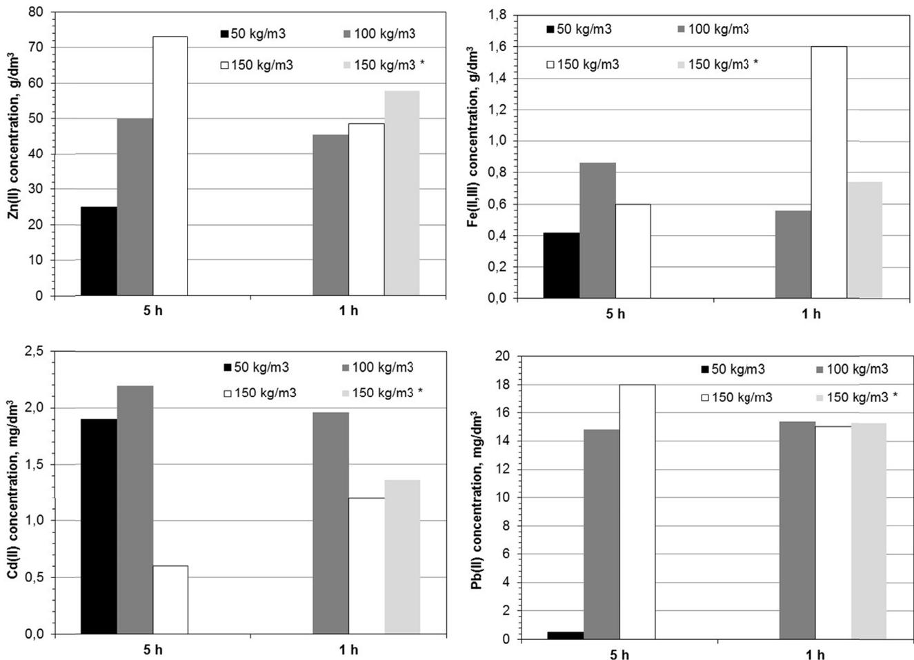
Fig. 4. Influence of the leaching time, bath loading and agitation rate (300 rpm and 900 rpm \*) on the final concentrations of metal ions in the solutions (20°C)
