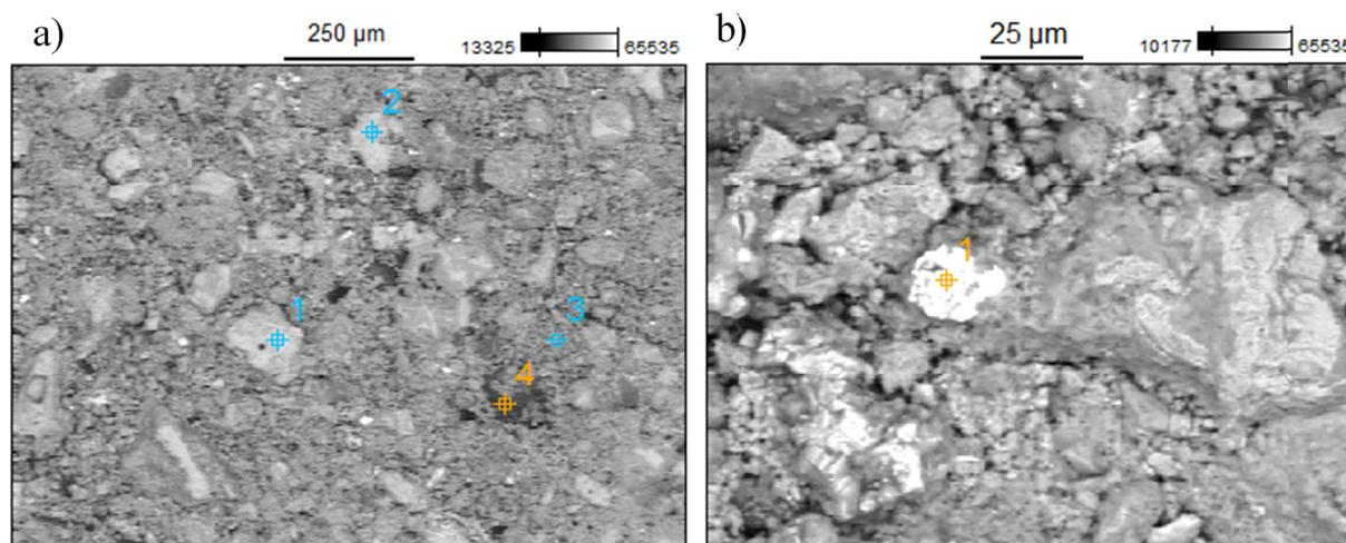
Fig. 1. Morphology of zinc ash oxide fraction
