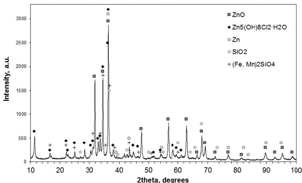
Fig. 2. Diffraction patterns of zinc ash
