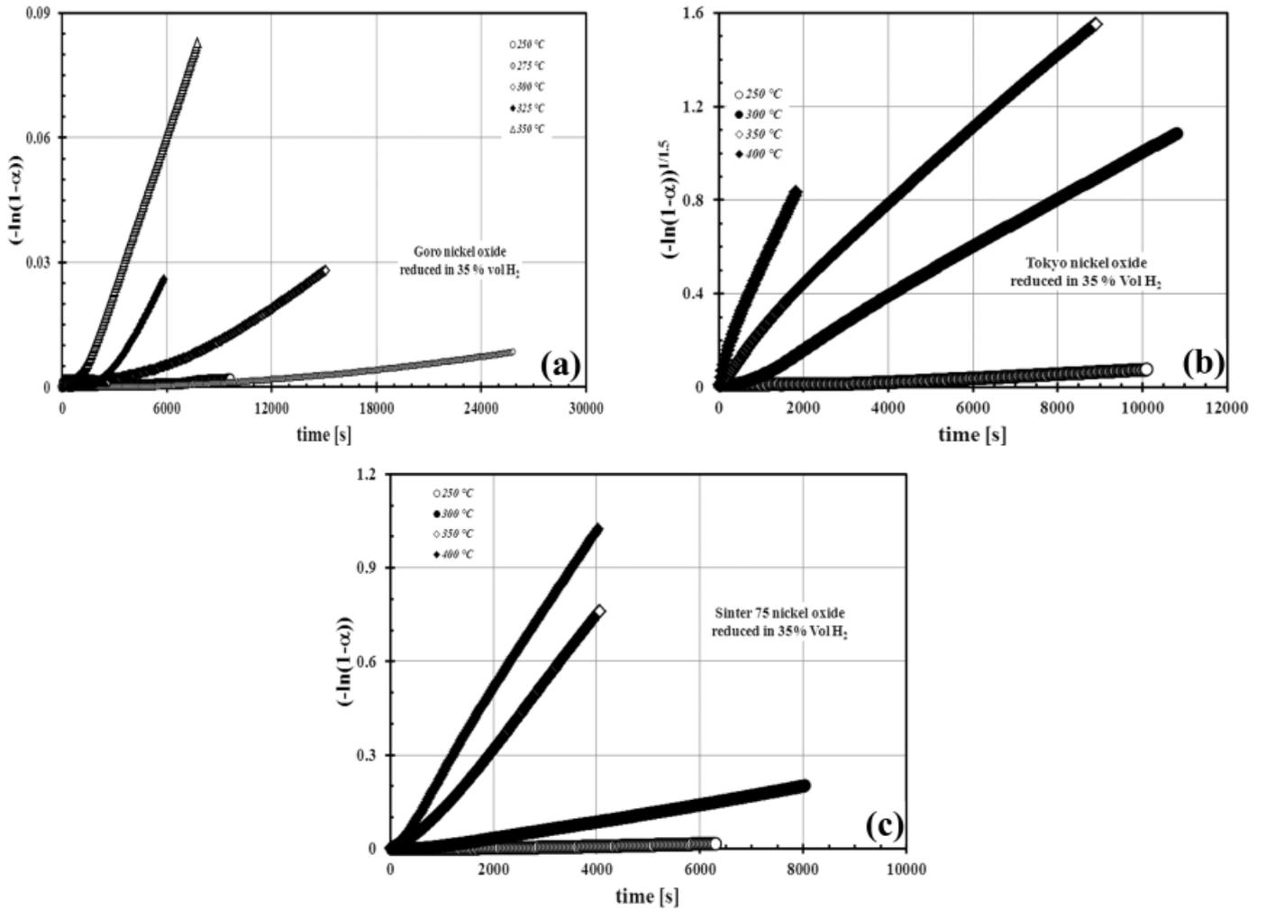
Fig. 7. Estimation of kinetic rate constants using the second order Avrami-Erofev kinetic model for (a) Goro oxide, (b) Tokyo oxide and (c) Sinter 75 oxide
