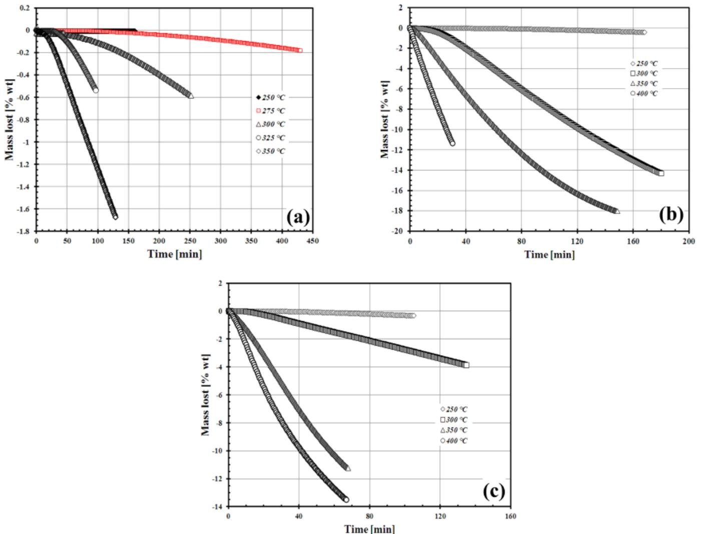
Fig. 2. Nickel oxide mass lost (wt%) as a function of time between 523 and 673 K (250 and 400°C) in a gas containing 35%vol H<sub>2</sub> for (a) Goro nickel oxide, (b) Tokyo nickel oxide and (c) Sinter 75 nickel oxide
