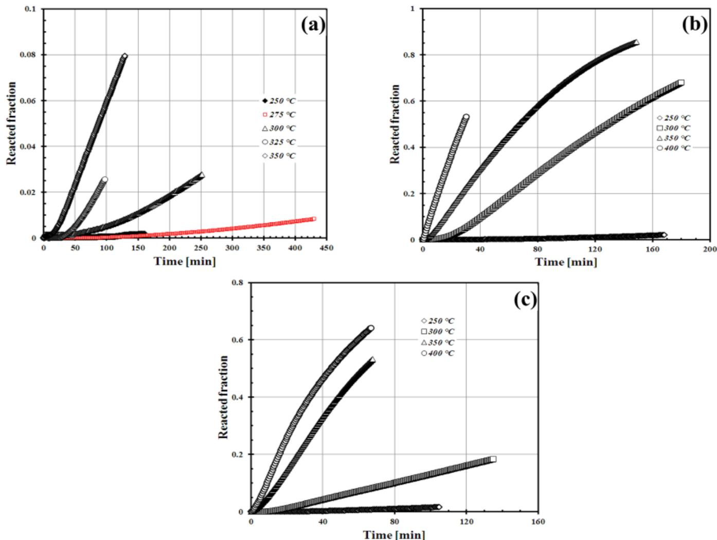
Fig. 3. Reacted fraction during the reduction between 523 and 673 K (250 and 400°C) in a gas containing 35%vol H<sub>2</sub> of (a) Goro oxide, (b) Tokyo oxide and (c) Sinter 75 oxide
