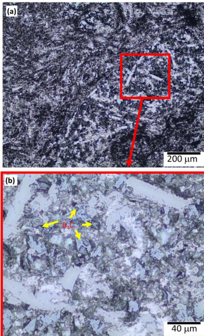
Fig. 1. Optical micrograph of the microstructure of the rapidly solidified Al-20Si-5Fe-15B<sub>4</sub>C metal matrix compounds after hot pressing
