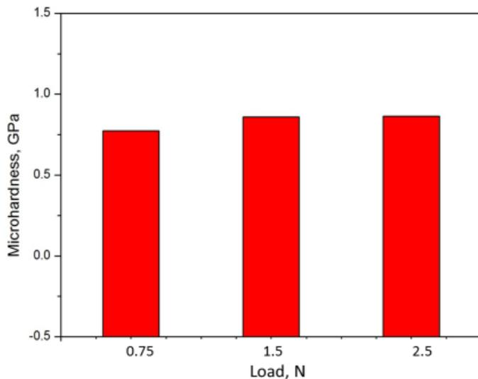
Fig. 4. Microhardness values calculated using Oliver-Pharr approach from the loading-unloading data under different peak loads
