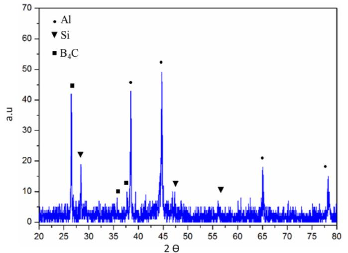
Fig. 2. The X-ray diffraction pattern of compacted B<sub>4</sub>C reinforcement melt – spun Al-20Si-5Fe alloy metal matrix composite
