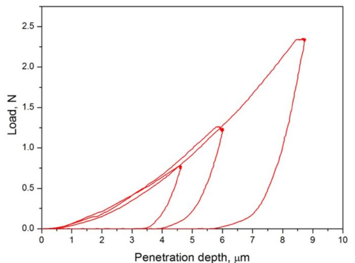
Fig. 3. Loading – unloading curves of rapidly solidified Al-20Si-5Fe-15B<sub>4</sub>C metal matrix composite obtained from indentation tests
