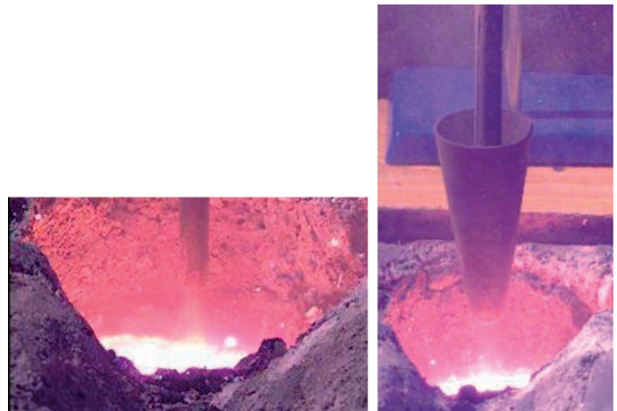
Fig. 6. Gas-ferroalloy particles penetration into liquid cast iron: left – simple steel lance for p_1 = 0,2\text{MPa} i p_4 = 0,08\text{MPa} , right – new lance with a flange p_1 = 0,2\text{MPa} i p_4 = 0,14\text{MPa}
