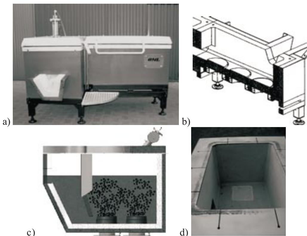
Fig. 1. URC-7000 reactor: a) real view, b) section through the refining chamber with the ceramic porous plugs, c) simulation of gas dispersion in the chamber, d) filter and the filtration chamber [14,15]
