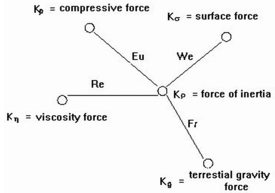
Fig. 3. The graphical presentation of forces creating dimensionless criterial numbers [22]
