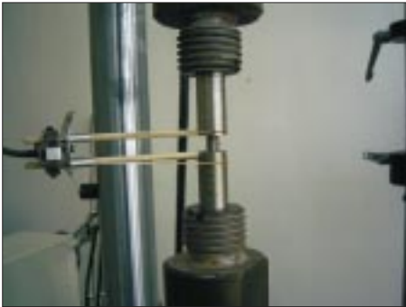
Fig. 2. Sintered sample between Instron push – rods equipped with high – temperature extensometr
