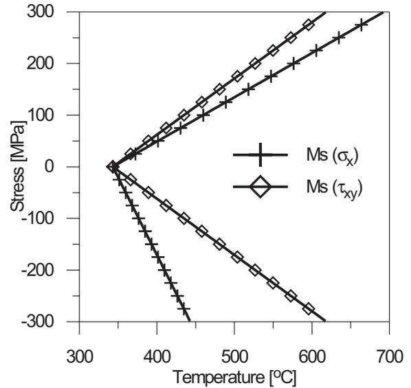
Fig. 5. Influence of stresses (normal  $\sigma_x$  and tangential  $\tau_{xy}$ ) on martensite start temperature ( $M_s$ )
