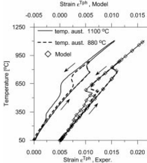
Fig. 7. Influence of austenitisation temperature on the dilatometric curves. (Experimental researches and numerical simulations)
