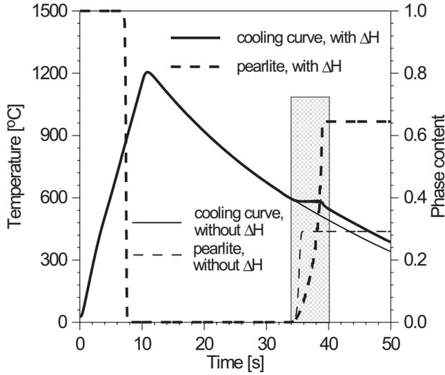
Fig. 2. Influence of latent heat of transformation on kinetic of phase transformation in the volumetric hardening, the middle node of cubical steel element
