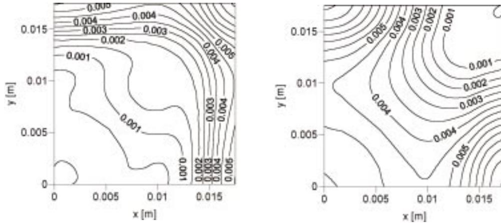
Fig. 13. The effective plastic strains: a) cross-sections, b) external surface
