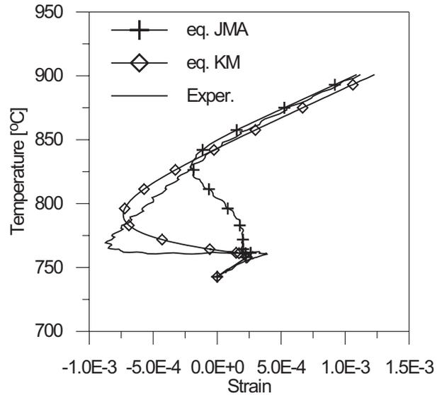
Fig. 4. The strains during austenite formation for heating rate  $100^{\circ}\text{C/s}$
