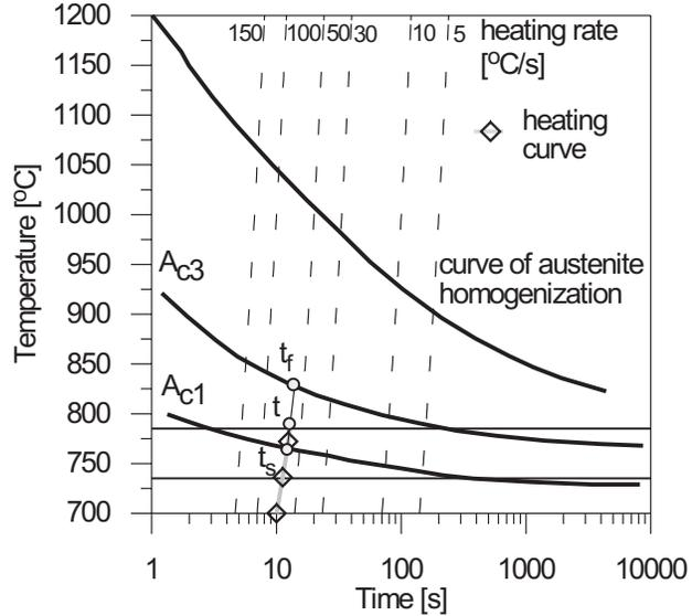
Fig. 3. The analysis of the diagram CHT, steel C45
