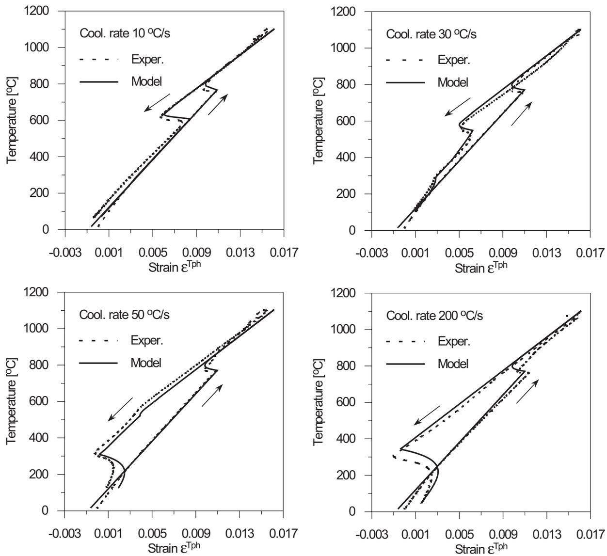
Fig. 8. Experimental and simulated dilatometric curves: a) 10°C/s, b) 30°C/s, c) 50°C/s, d) 200°C/s
