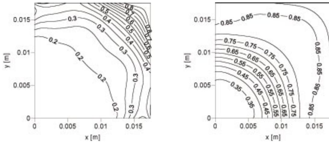
Fig. 10. The field of martensite: a) cross-sections, b) external surface
