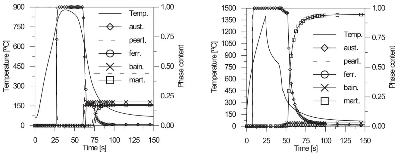
Fig. 9. The kinetics of phase transformations and temperature: a) in the middle node, b) in the corner node
