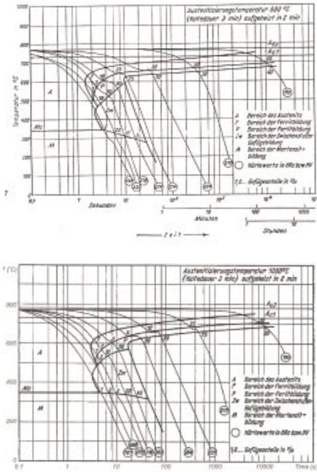
Fig. 6. The CCT diagrams of the C45 steel for different austenitisation temperatures: a) 880°C [16], b) 1050°C [17]
