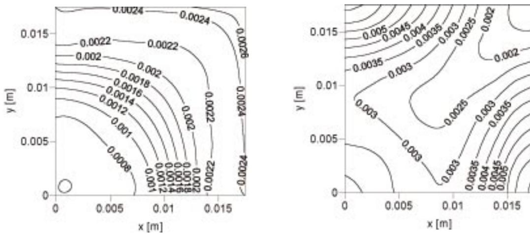
Fig. 11. The strains on external surface: a) the structural strains, b) the effective transformations plasticity
