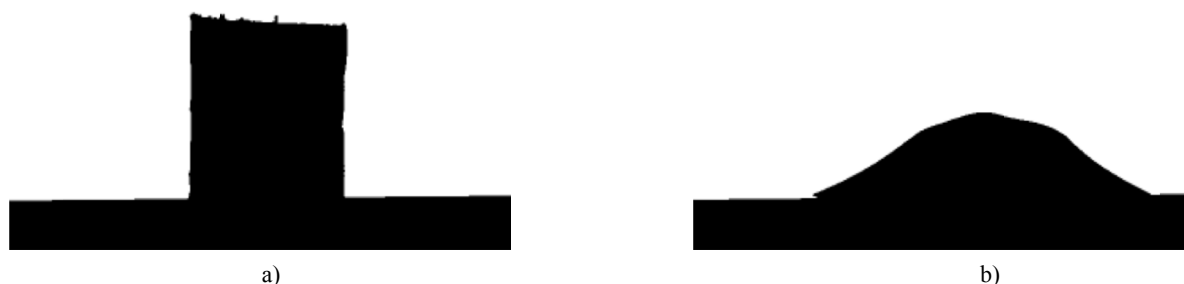
Fig. 4. The result of measurements with a high-temperature microscope for mould flux 2, taken in the second minute after being fed into the mould, a) temp. 920°C, b) temperature 1136°C
