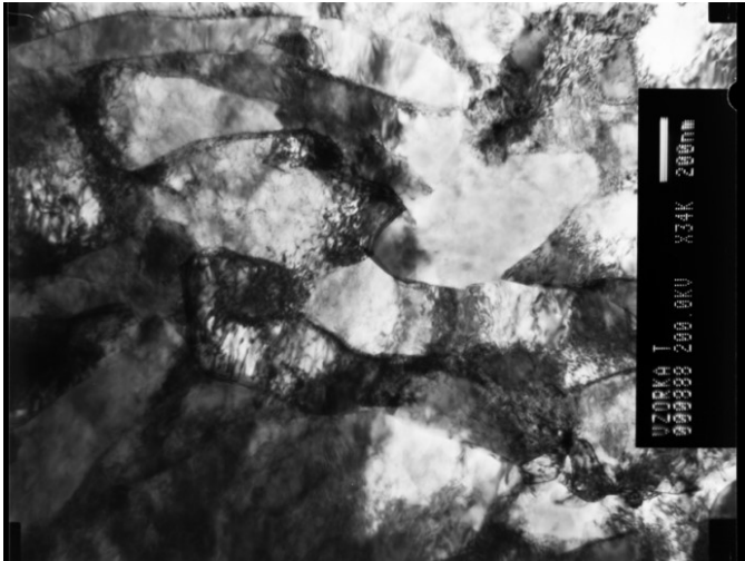
Fig. 4. TEM image of OFHC copper after five ECAP passes
