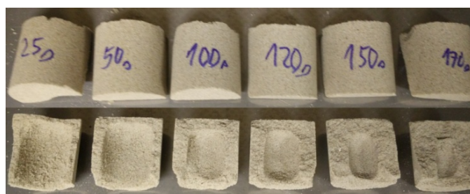
Fig. 1. Shell formation in dependence of curing time (from left 25, 50, 100, 120, 150, 170 seconds)
