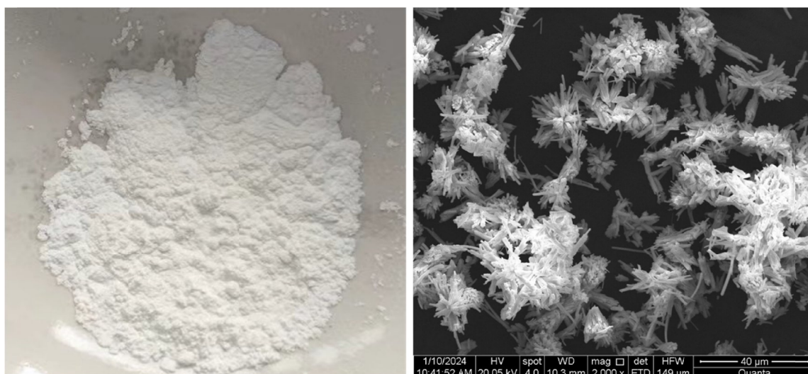
Fig. 13. SEM-mapping images of the yttrium oxide product
