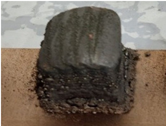
Fig. 2. Deposition of gradient path FGM block based on first experimental parameter set
