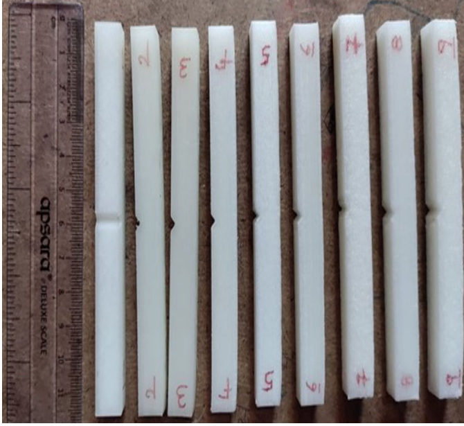
Fig. 4. Printed specimens for Charpy impact test as per the experimental design
