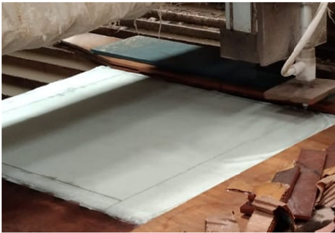
Fig. 2. Waterjet cutting of laminates
