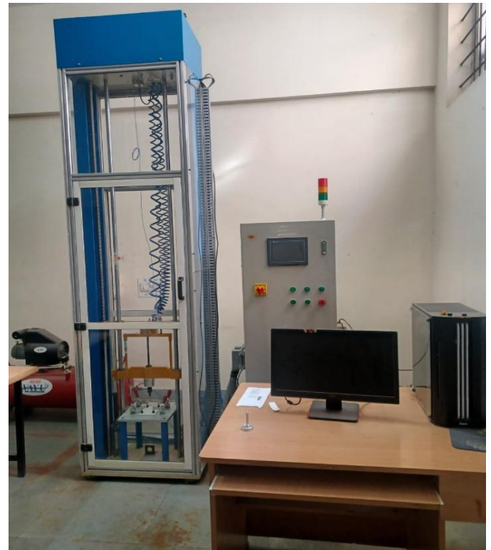
Fig. 3. Low velocity impact testing machine
