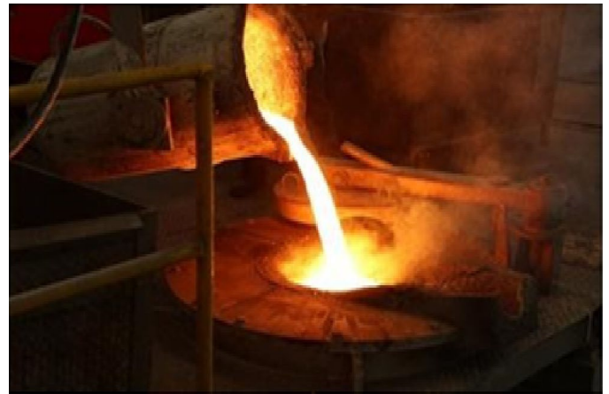
Fig. 1. Iron melting induction furnace Stir Casting of Nanocomposites
