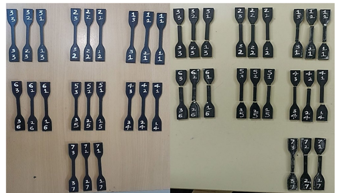
Fig. 3. Tensile test samples before and after testing
