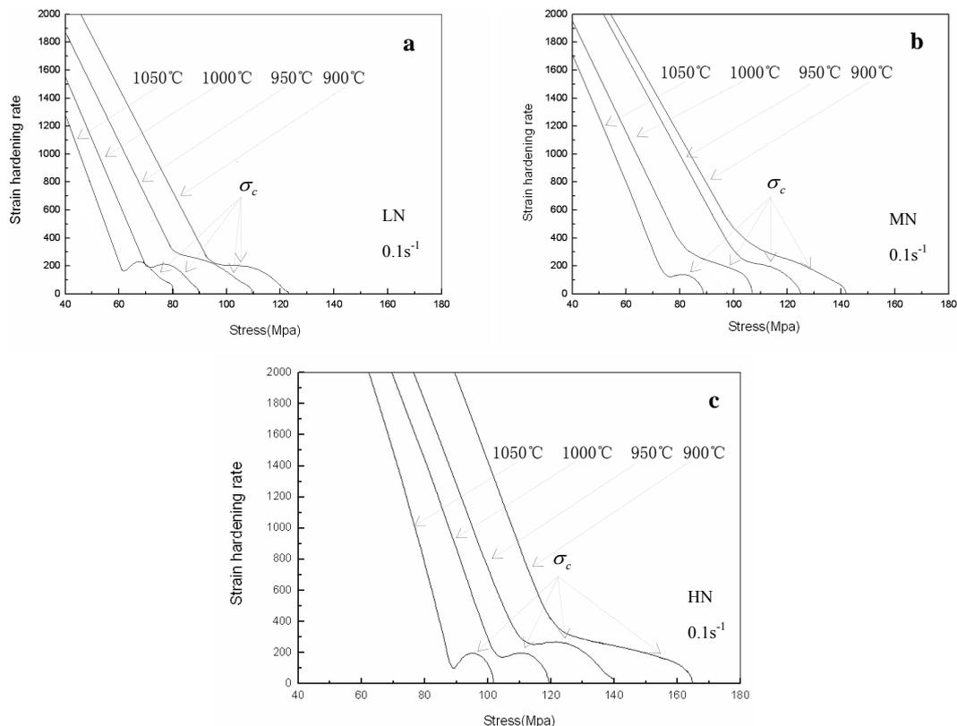
Fig. 3. Strain hardening versus stress curves of the tested steel (a) low nitrogen steel (b) medium nitrogen steel (c) high nitrogen steel
