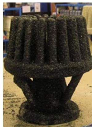
Fig. 1. The pattern assembly with 20 airfoil blade castings
