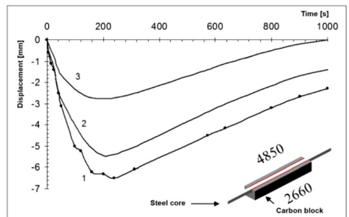
Fig. 6. Changes in the displacement of pin ends during cooling of cast iron in the shaped groove examined for the section preheated to a temperature of  $T_N = 200^\circ\text{C}$  and  $T_N = 350^\circ\text{C}$ ; 1 – the displacement determined empirically for  $T_N = 200^\circ\text{C}$ , 2 – the displacement determined numerically for  $T_N = 200^\circ\text{C}$ , 3 – the displacement determined empirically for  $T_N = 350^\circ\text{C}$ .
