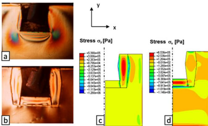
Fig. 5. Stresses visible in the zone of angular cracks after the lapse of 30 seconds since the time instant of filling the shaped groove with cast iron; a – the original design; elasto-optic image y, b – the design after modifications; elasto-optic image, c, d – the design after modifications; numerical calculations
