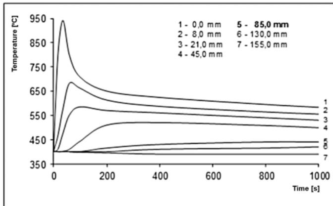
Fig. 2. Temperature changes in the cross-section of carbon block at different distances from the surface of the shaped groove.
