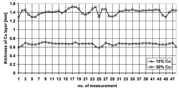
Fig. 8. Distribution of Cu layer thickness over the aluminium core after the final pass: a) Al-Cu – 15% Cu, b) Al-Cu – 30%Cu
