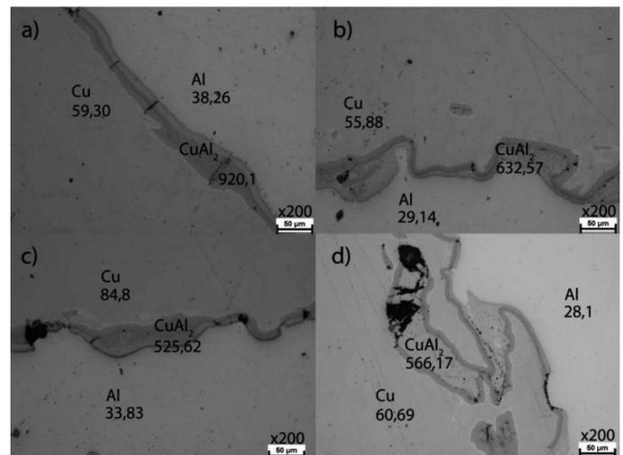
Fig. 10. The results of  $HV_{0.05}$  microhardness measurements in the connection areas: a) sample no. 1, 15% Cu – after first pass, b) sample no. 9, 30% Cu – after first pass; c) sample no. 1, 15% Cu, after the final pass, d) sample no. 9, 30% Cu, after the final pass
