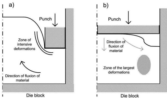
Fig. 1. Schematic of the alternate extrusion and multiaxial compression process; a) extrusion operation; b) compression operation
