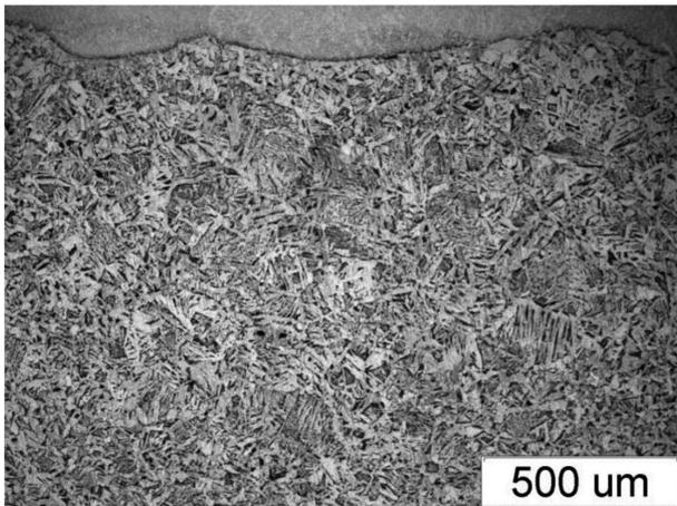
Fig. 2. High amount of acicular ferrite in weld (71%) after Ar/CO<sub>2</sub> micro-jet cooling
