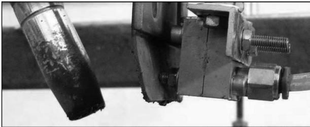
Fig. 1. Montage of welding head and micro-jet injector
