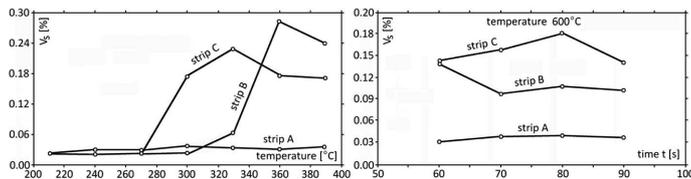
Fig. 5. Progress in the recrystallisation of clad strips
