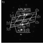
Fig. 3. Structure of the thin foil from the (Al,Ti)N coating: a) bright field; b) diffraction pattern from area a and solution of the diffraction pattern
