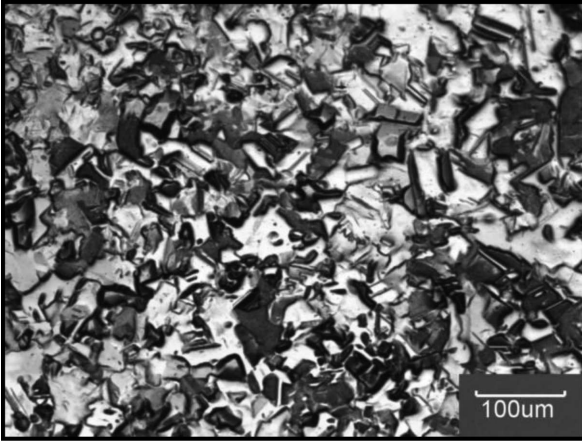
Fig. 3. Optical photomicrograph of copper
