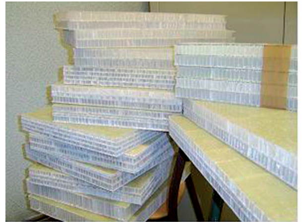
Fig. 3. Honeycomb multi-layer sandwich
