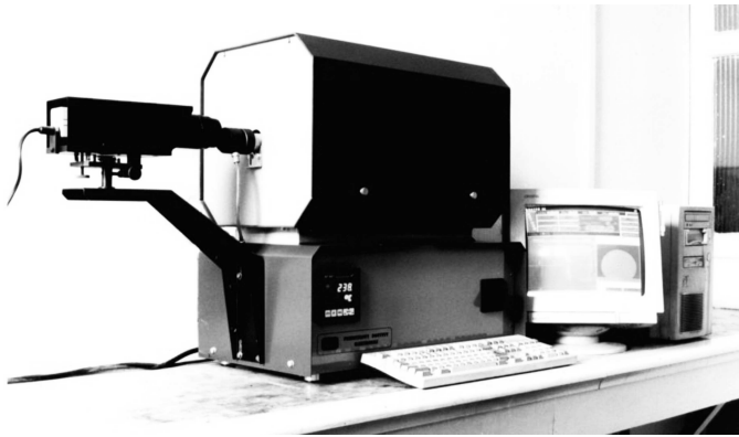
Fig. 1. A high-temperature microscope applied in the measurements of liquid Cu-Ag alloy surface tension
