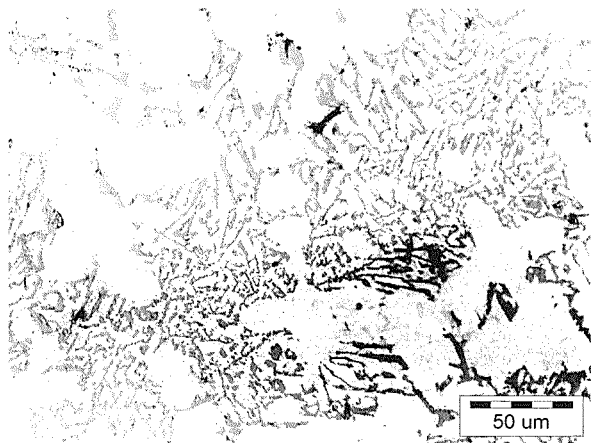
Fig. 5. Microstructure of the Al-12Si alloy with 0.6 at.% addition of the Al-12Si modifier cooled at the rate: 200 K/s
