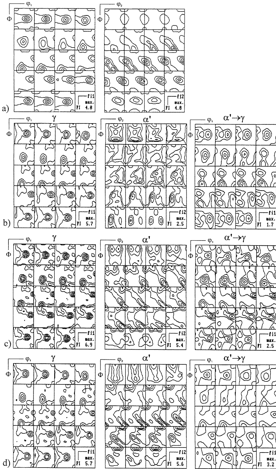
Fig. 4. Orientation distribution functions (ODF) of AISI 302 steel: (a) for the austenite after solution treatment, for the austenite ( \gamma ), martensite ( \alpha ) and after transformation \alpha' \rightarrow \gamma - (b) 37.4%, (c) 70.6%, (d) 91.6%
