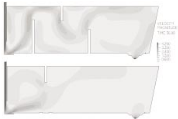
Fig. 7. Distribution of velocity magnitude at t = 36 s for initial (top) and final (bottom) solution
