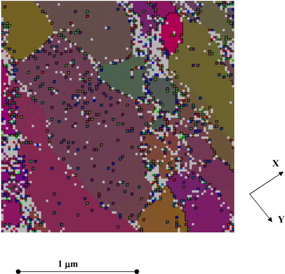
Figure 3 :b) Orientation map build with CBED patterns of an Aluminum sample deformed by ECAE.
