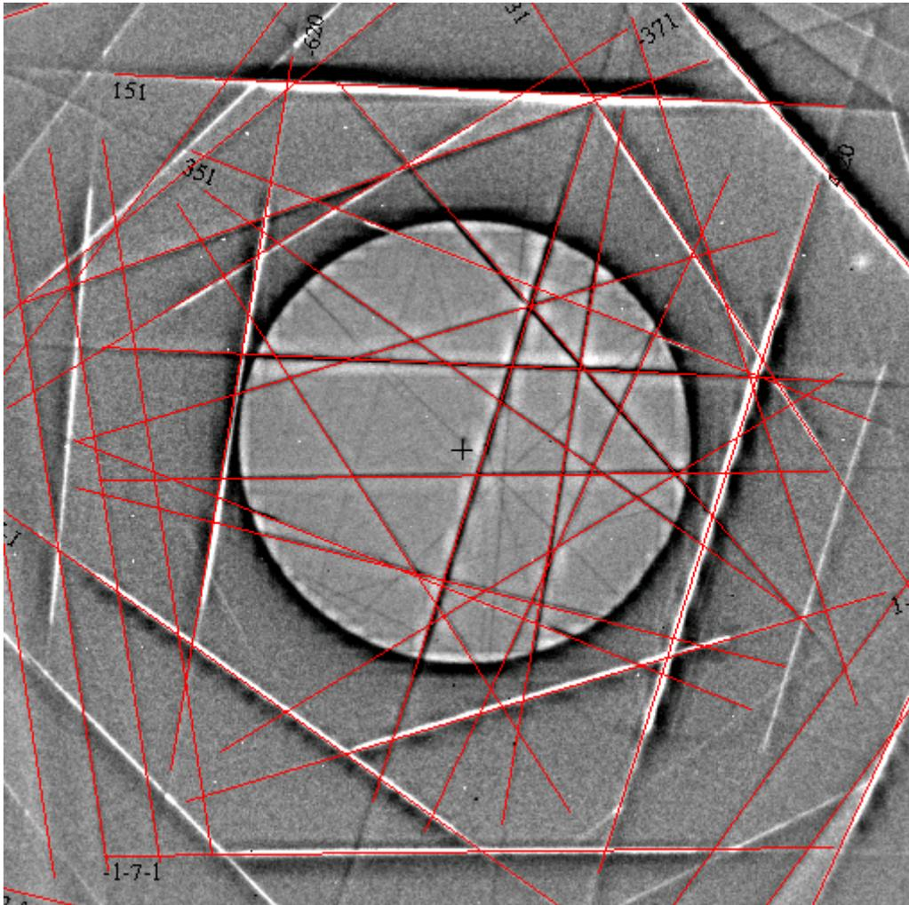
Figure 3 : a) Orientation map build with Kikuchi patterns of an Aluminum sample deformed by ECAE.
