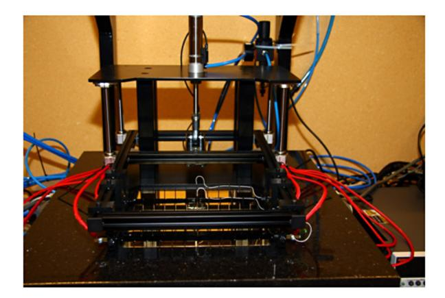
Fig. 4. Measuring table with the multi-pin voltage/current probes of the setup (Fig.3).
