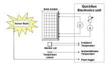
Fig. 1. The scheme of the measurement system - simulator for
