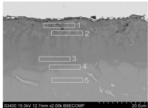
Fig. 1. Structure of aluminide coating deposited by VPA method on  $\gamma$ -TiAl intermetallic alloys
