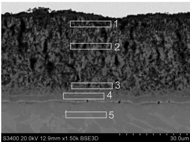
Fig. 3. Microstructure of aluminate coating deposited by pack cementation method on TiAl intermetallic alloy
