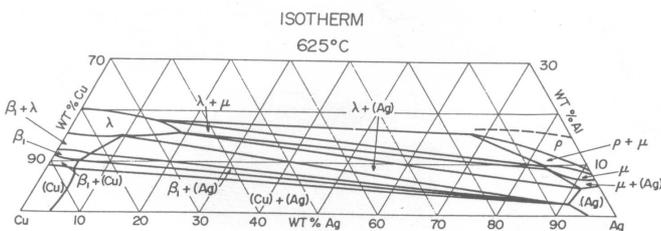
Fig. 1. Isothermal cross-section at 898K of part of the equilibrium system of Ag-Cu-Al [8]
