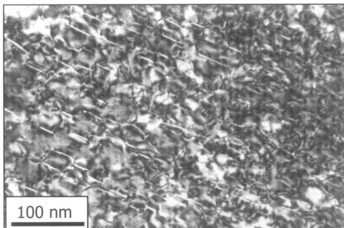
Fig. 5. Microstructure of AgCuAlGa alloy aged at 523K for 90 minutes
