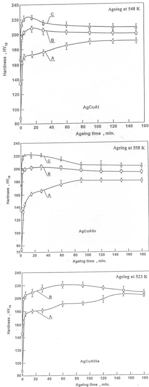
Fig. 3. Changes in the hardness HV10 with the duration of ageing of AgCuAl, AgCuAlIn, AgCuAlGa alloys after: 1) solution heat treatment, 2) solution heat treatment and deformation by  $\epsilon = 30\%$ , 3) solution heat treatment and deformation by  $\epsilon = 60\%$
