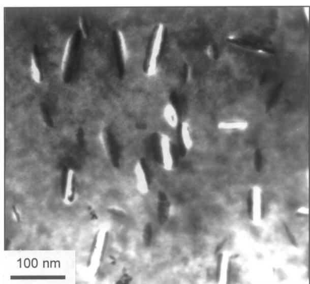
Fig. 7. Microstructure of AgCuAlGa alloy aged at 523K for 180 minutes
