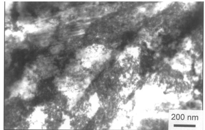
Fig. 12. Microstructure of AgCuAlGa alloy solution heat treated and deformed by  $\epsilon = 30\%$  and next aged at 523K for 80 minutes
