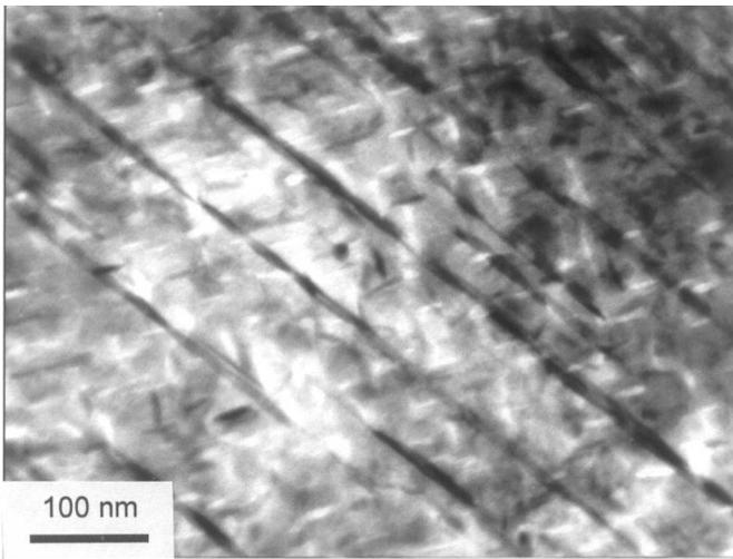
Fig. 9. Microstructure of AgCuAlIn alloy solution heat treated and deformed by  $\epsilon = 30\%$  and next aged at 558K for 30 minutes
