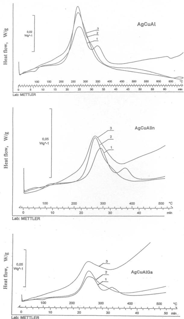
Fig. 2. Calorimetric curves of the alloys: AgCuAl, AgCuAlIn, AgCuAlGa after: 1) solution heat treatment, 2) solution heat treatment and deformation by  $\epsilon = 30\%$ , 3) solution heat treatment and deformation by  $\epsilon = 60\%$
