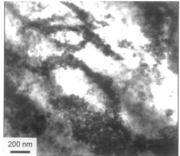
Fig. 11. Microstructure of AgCuAl alloy solution heat treated and deformed by  $\epsilon = 30\%$  and next aged at 548K for 60 minutes
