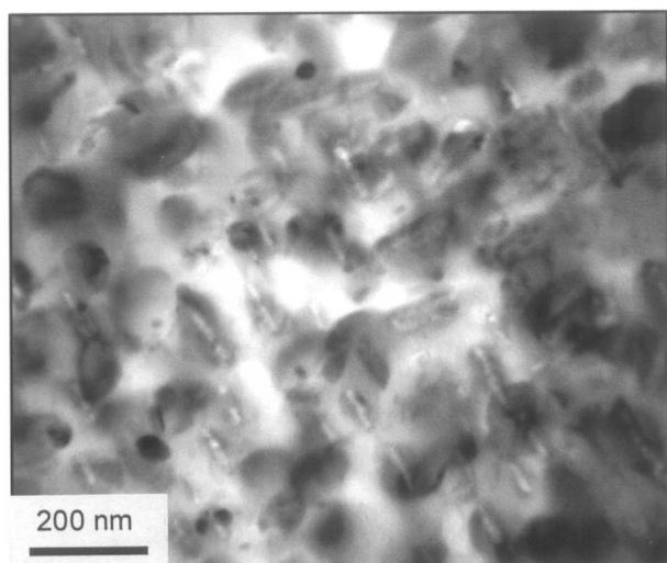
Fig. 6. Microstructure of AgCuAlIn alloy aged at 558K for 140 minutes
