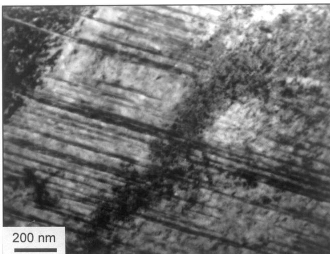
Fig. 10. Microstructure of AgCuAlGa alloy solution heat treated and deformed by  $\epsilon = 30\%$  and next aged at 523K for 80 minutes
