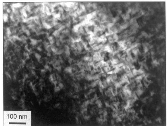
Fig. 4. Microstructure of AgCuAlIn alloy aged at 558K for 90 minutes
