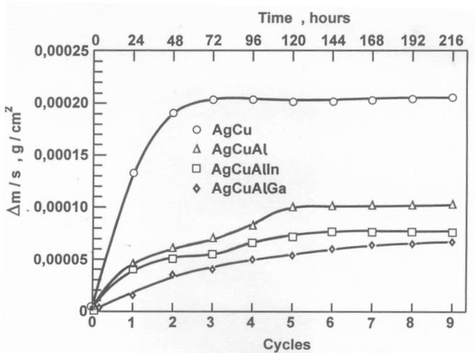
Fig. 13. Elementary mass changes of AgCuAl, AgCuAlIn, AgCuAlGa alloys and the jewellery alloy AgCu7.5 as a function of the cycle (duration) during the corrosion resistance in humid atmosphere, containing SO<sub>2</sub>
