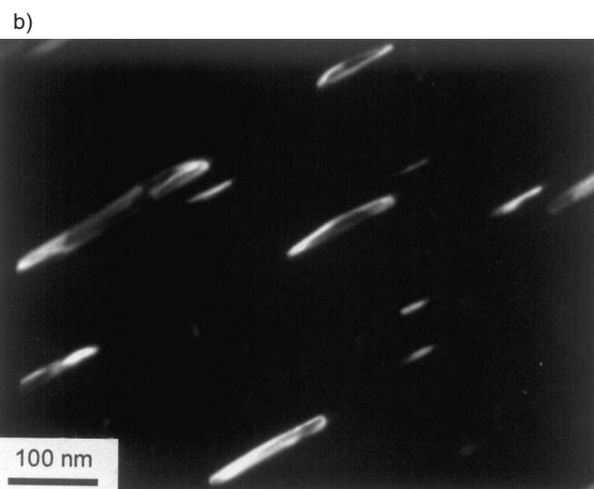
Fig. 8. Microstructure of AgCuAlIn alloy aged at 558K for 1400 minutes, a) observation in a bright field, b) observation in a dark field
